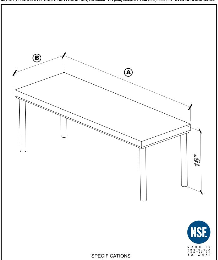
STA - PRO TS - 1 SERIES TABLE SHELVES ARE CONSTRUCTED OF 16 GAUGE T -304 STAINLESS STEEL WITH A # 4 FINISH. EDGES ARE TURNED DOWN 1.75". POSTS ARE 1" O.D. STAINLESS STEEL TUBE WITH INTERNAL THREADED FASTENERS AT THE BOTTOM TO ALLOW BOLTING SHELF TO TABLE TOPS FROM BELOW. SHELF IS REINFORCED WITH S/S HAT CHANNELS. OPTIONAL MOUNTING PADS OR SPECIAL BRACKETS CAN BE SUPPLIED. SPECIFY THE LENGTH (A) AND THEN THE SERIES REQUIRED FOLLOWED BY THE FRONT TO BACK (B) MEASUREMENT.
