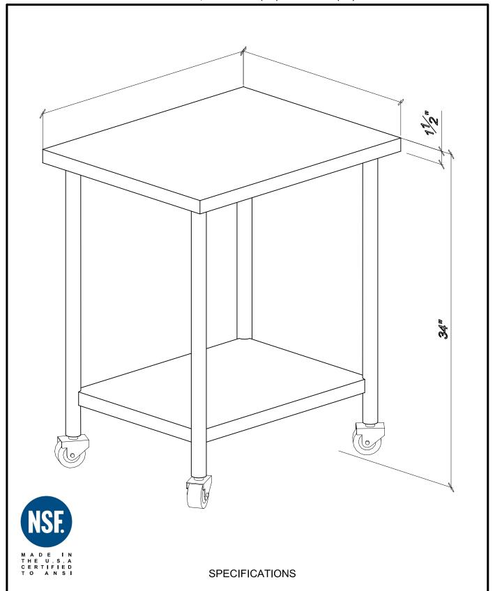
STA-PRO #SST MOBILE UTILITY TABLES ARE CONSTRUCTED WITH A FULL PERIMETER ANGLE IRON FRAME TO SUPPORT THE 16 GA. TYPE #504 STAINLESS STEEL TUBE FITTED WITH FOUR (4) 5" DIAMETER HEAVY DUTY BALL BEARING SWIVEL CASTERS, WITH NON-MARKING RUBBER TIRES, TWO (2) CASTERS FITTED WITH BRAKES, THE 18 GA. STAINLESS STEEL UNDERSHELF IS REINFORCED WITH 16 GA. CHANNEL AND FULLY WELDED AT EACH LEGS 8" ABOVE FLOOR.
